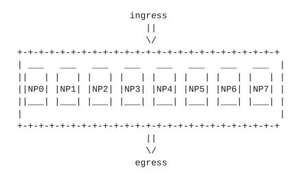
To assign incoming traffic to the various NPs, suppose a hashing algorithm performs an exclusive-or (XOR) operation on the least significant 3 bits of the source and destination MAC addresses in each frame. (This is an actual example the authors have observed in multiple devices from multiple manufacturers.)
