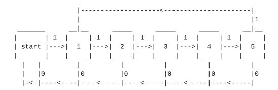
Initially, we begin in the "start" state. A 1 bit moves us into the next highest state, and a 0 bit returns us to the start state. From state 5, a 1 bit takes us back to the 1 state and a 0 bit returns us to "start." From this state table we can build the following transition matrix:
