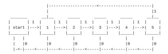
Initially, we begin in the "start" state. A "1" bit moves us into the next highest state, and a "0" bit returns us to the start state. From state 5, a "1" bit takes us back to the 1 state and a "0" bit returns us to "start."
