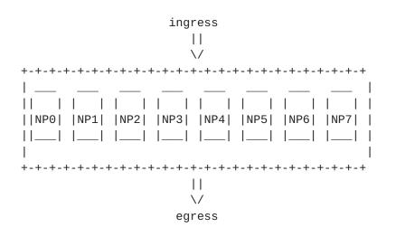
To assign incoming traffic to the various NPs, suppose a hashing algorithm performs an exclusive-or (XOR) operation on the least significant 3 bits of the source and destination MAC addresses in each frame. (This is an actual example the authors have observed in multiple devices from multiple manufacturers.)
