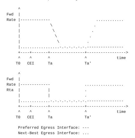
With TO the Start Traffic Instant; CEI the Convergence Event Instant; Ta the time instant packet loss for route Rta starts; Ta' the time instant packet impairment for route Rta ends.
