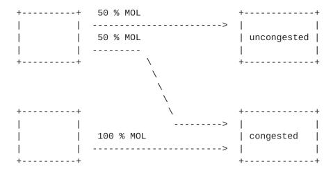
Both source transmitters MUST transmit the exact number of frames. The first source MUST transmit frames at the MOL with the destination address of the two receive ports in an alternating order. The first frame to the uncongested receive port, second frame to the congested receive port, then repeat. The second source transmitter MUST transmit frames at the MOL only to the congested receive port.
