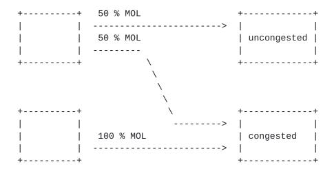
Both source transmitters MUST transmit the exact number of test frames. The first source MUST transmit test frames at the MOL with the destination address of the two receive ports in an alternating order. The first test frame to the uncongested receive port, second test frame to the congested receive port, then repeat. The second source transmitter MUST transmit test frames at the MOL only to the congested receive port.
