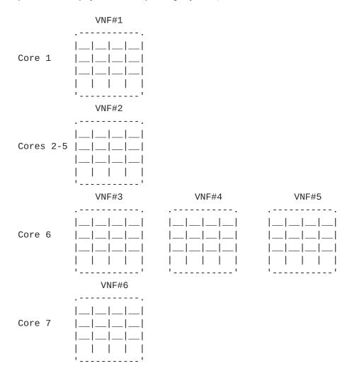
The combination of tables above could be built incrementally, beginning with VNF#1 and one Core, then adding VNFs according to their supporting core assignments. X-Y plots of critical benchmarks would also provide insight to the effect of increased HW utilization.
