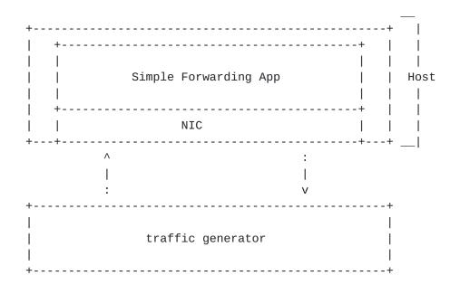
\* Benchmark VNF forwarding capability with direct connectivity (vSwitch bypass, e.g., SR/IOV) for at least 72 hours (serves as a means of VNF validation and a means to obtain the base performance for the VNF in terms of its maximum forwarding rate and latency). The metrics gathered from this test will serve as a key comparison point for vSwitch bypass technologies performance and vSwitch performance.
