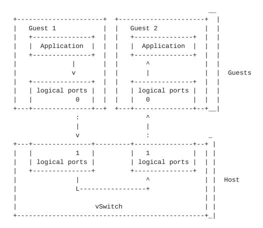
A set of Deployment Scenario figures is available on the VSPERF Test Methodology Wiki page [TestTopo].
