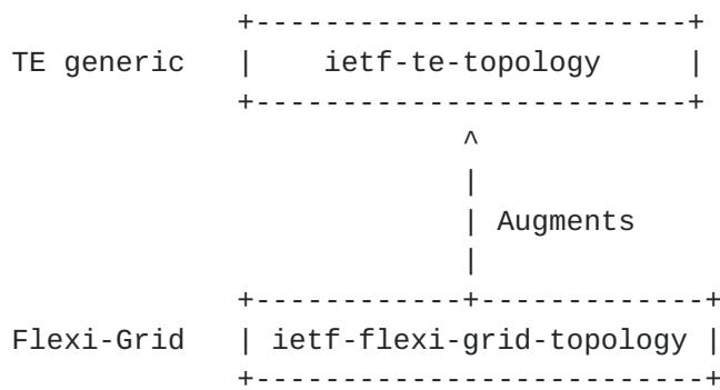
Figure 3: Relationship between Flexi-Grid and TE topology models
