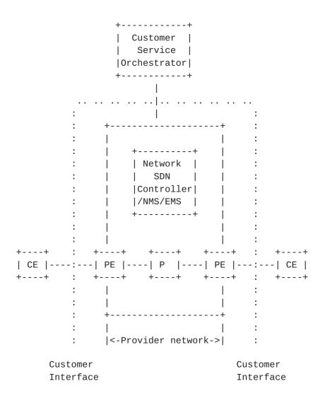
Figure 1: L1VPN SDN Controller/EMS/NMS-Based Service Model: External Customer
