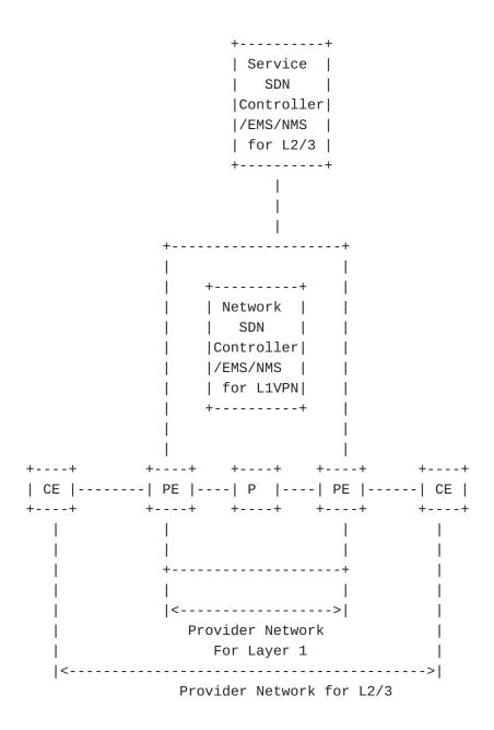
Figure 2: L1VPN SDN Controller/EMS/NMS-Based Service Model: Internal Customer
