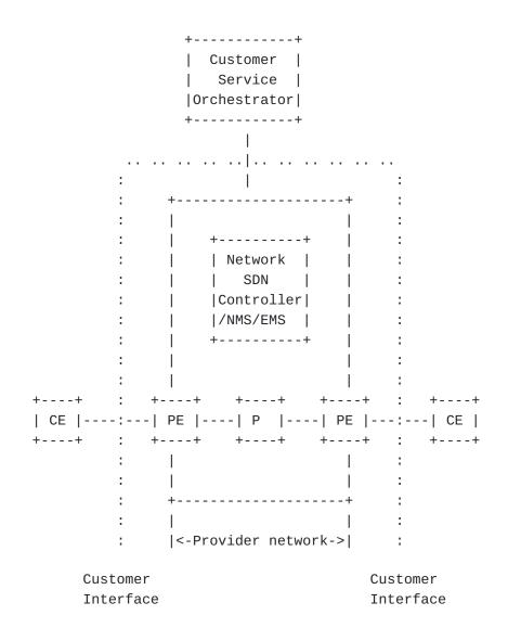
Figure 1: L1VPN SDN Controller/EMS/NMS-Based Service Model: External Customer
