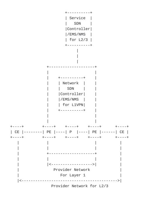
Figure 2: L1VPN SDN Controller/EMS/NMS-Based Service Model: Internal Customer
