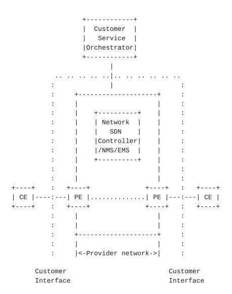
Figure 1: L1CSM SDN Controller/EMS/NMS-Based Service Model: External Customer
