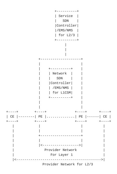
Figure 2: L1CSM SDN Controller/EMS/NMS-Based Service Model: Internal Customer
