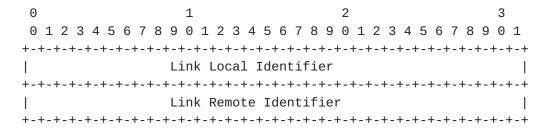
A node can communicate its Link Local Identifier to its neighbor using a link local Opaque LSA, as described in Section "Exchanging Link Local TE Information".
