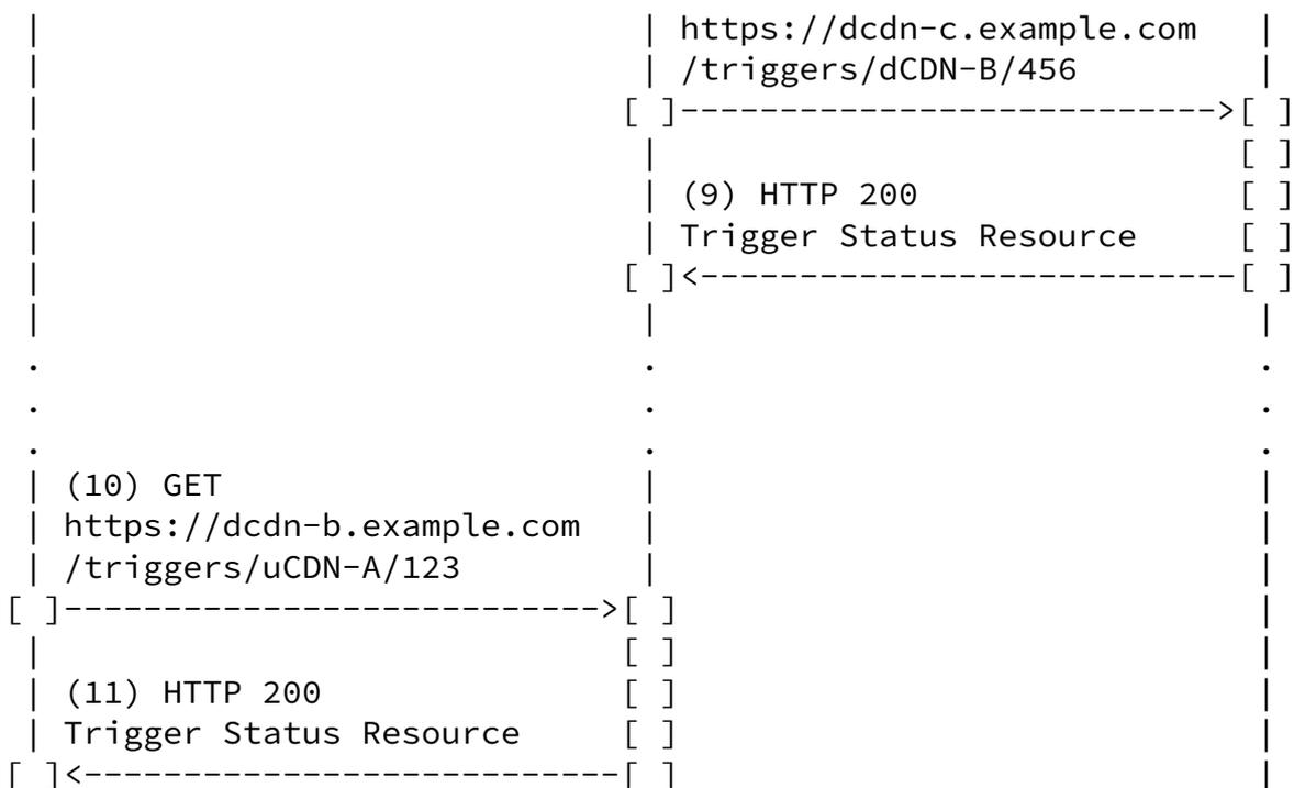
Figure 2: CDNI Message Flow for Triggers, Including Error Propagation
