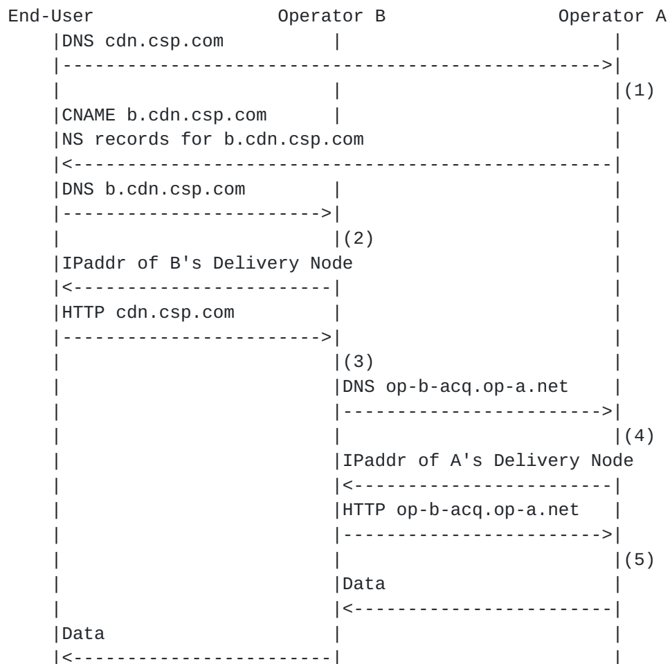
Figure 5: Request Trace for DNS-based Redirection Example
