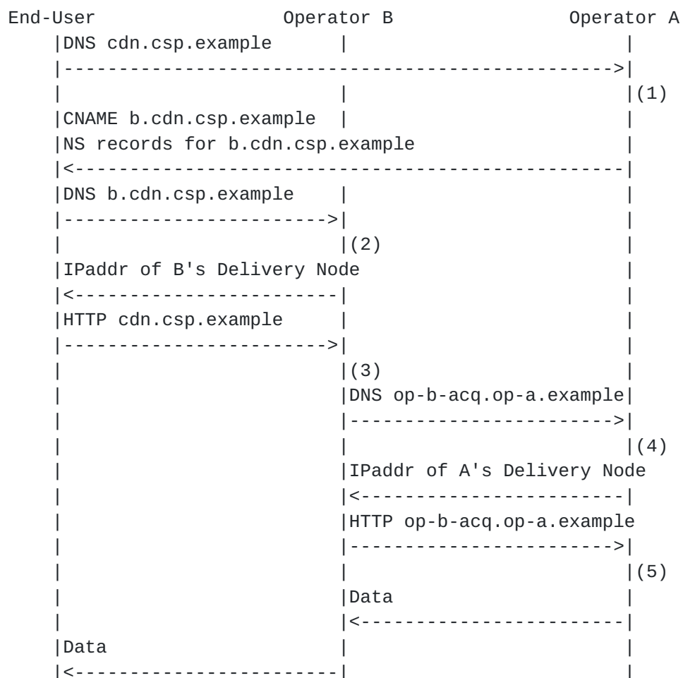
Figure 5: Message Flow for DNS-based Redirection
