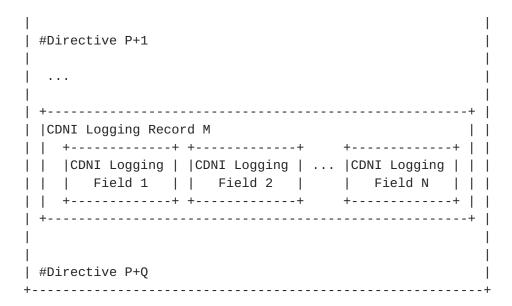
Figure 3: Structure of Logging Files
