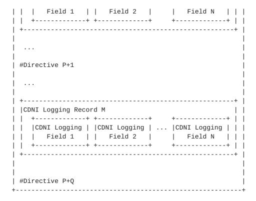
Figure 3: Structure of Logging Files
