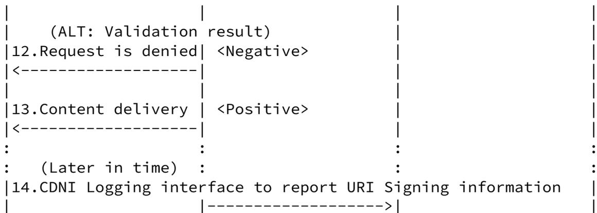
Figure 4: DNS-based Request Routing with URI Signing
