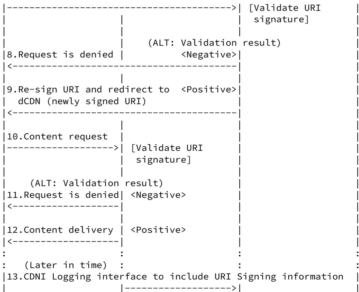
Figure 3: HTTP-based Request Routing with URI Signing
