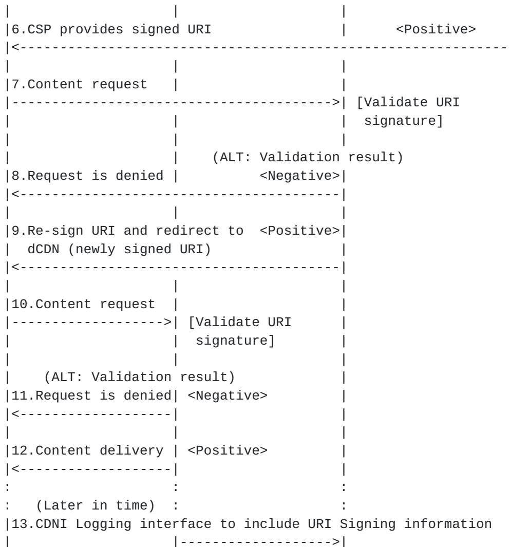
Figure 3: HTTP-based Request Routing with URI Signing
