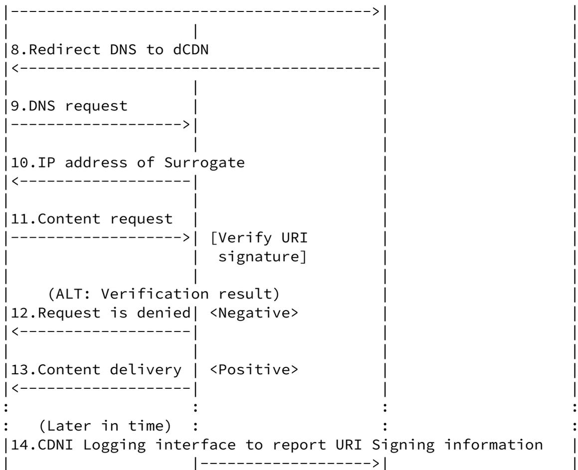
Figure 5: DNS-based Request Routing with URI Signing
