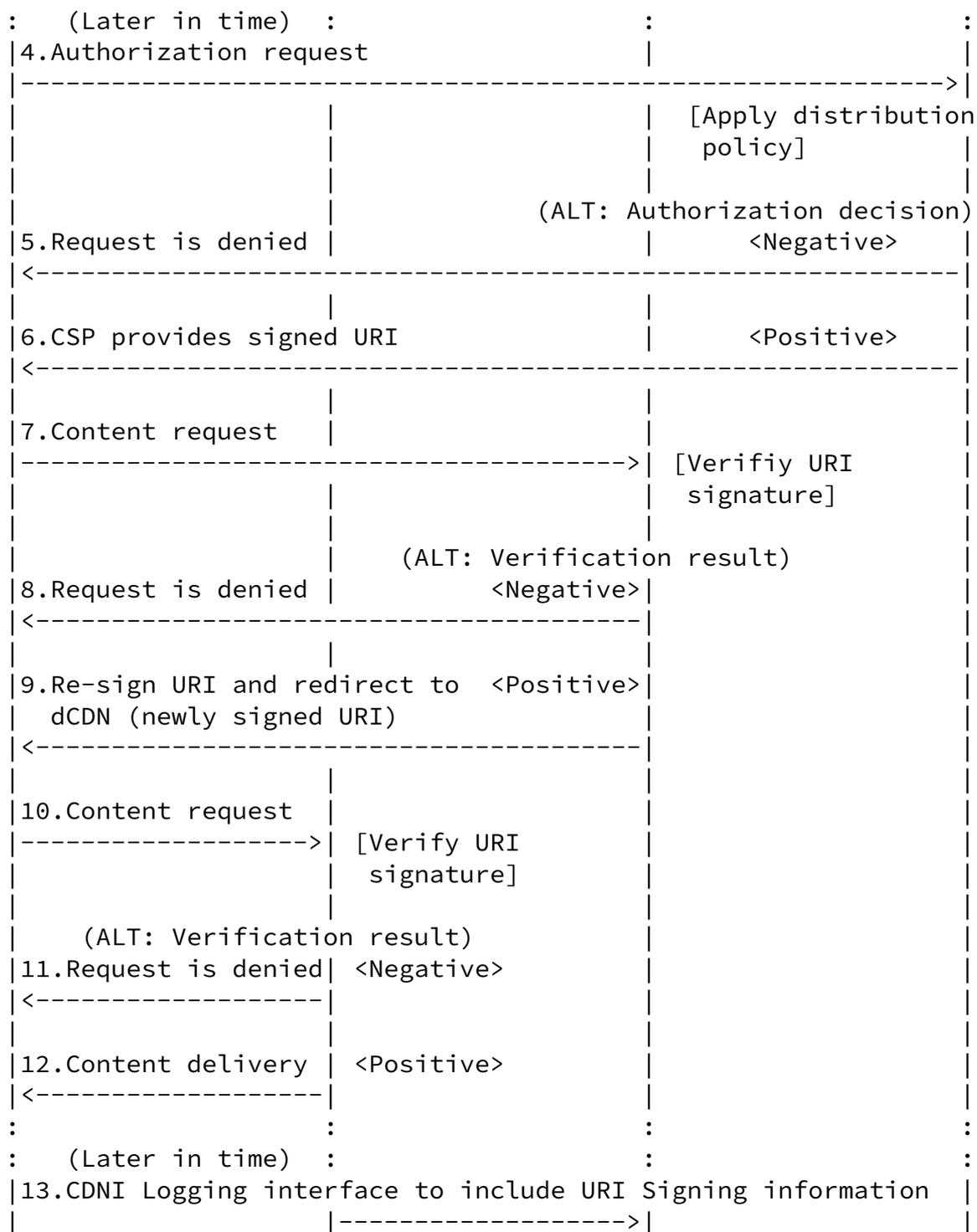
Figure 4: HTTP-based Request Routing with URI Signing
