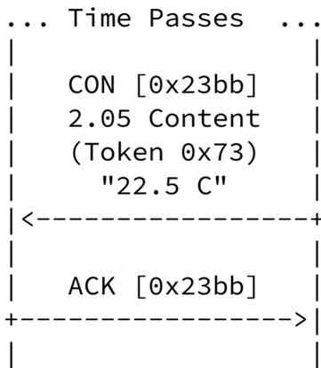
Figure 5: A GET request with a separate response
