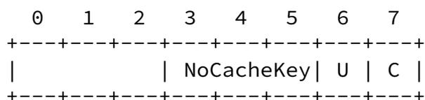
Figure 10: Option Number Mask (Least Significant Byte)
