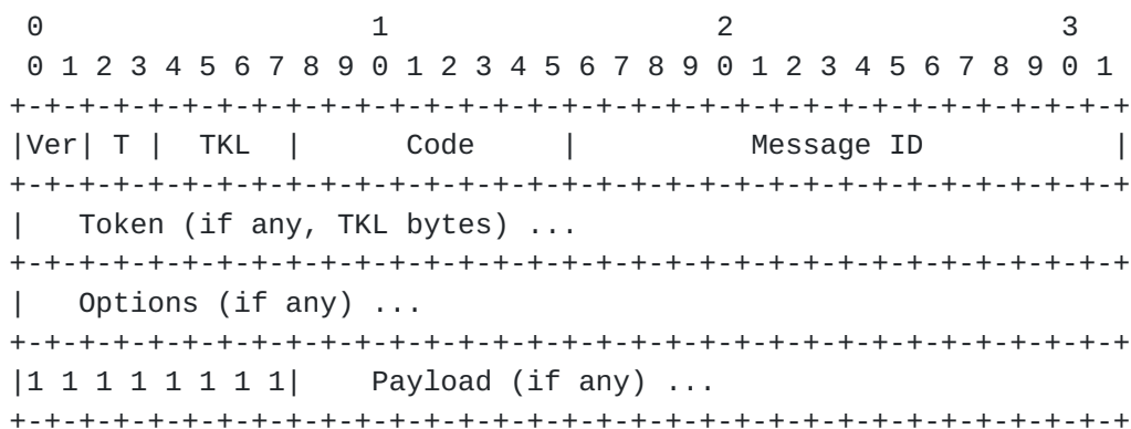
Figure 4: RFC 7252 defined CoAP Message Format.
