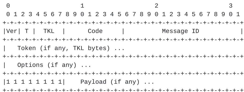
Figure 4: RFC 7252 defined CoAP Message Format.
