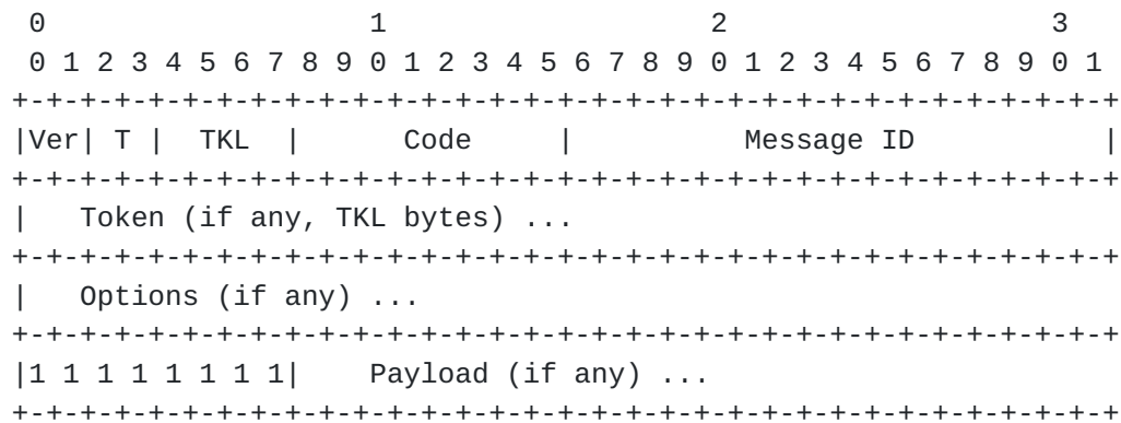
Figure 3: RFC 7252 defined CoAP Message Format
