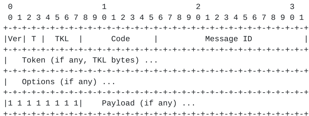
Figure 3: RFC 7252 defined CoAP Message Format
