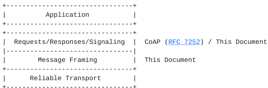
Figure 1: Layering of CoAP over Reliable Transports
