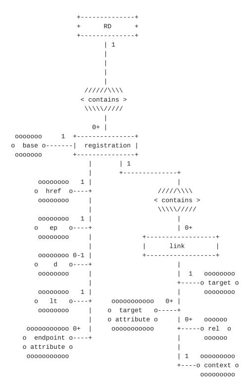
Figure 3: ER Model of the content of the RD
