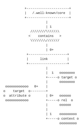
Figure 2: ER Model of the content of /.well-known/core
