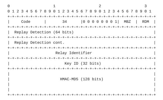
The suboption length is 34. The RDM and Replay Detection fields are as specified in <u>Section 5</u>. The Relay ID field is set as specified in <u>Section 6</u>. The Key ID is set by the sender to the ID of the key used in computing the signature, as an integer value in network byte-order. The HMAC signature follows the Key ID.
