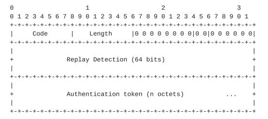
The authentication token is an opaque, unencoded value known to both the sender and receiver. The sender inserts the authentication token in the DHCP message and the receiver matches the token from the message to the shared token. If the authentication option is present and the token from the message does not match the shared token, the receiver MUST discard the message.
