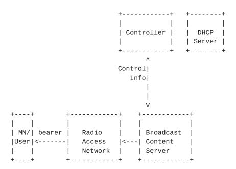
Note that this figure is shown here for broad understanding of how Broadcast and Multicast service works in a 3G cellular telehone network. The network elements except MN/user and the DHCP server are not relevant to the text in this document.
