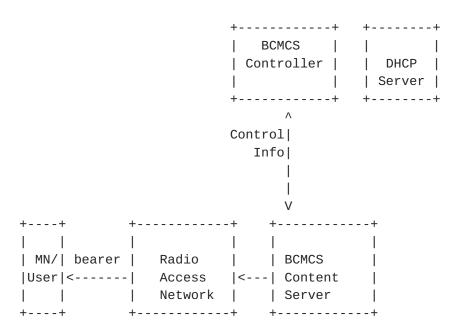
Note that this figure is shown here for a basic understanding of how Broadcast and Multicast service works in a 3G cellular telephone network. The network elements except MN/user and the DHCP server are not relevant to the text in this document.
