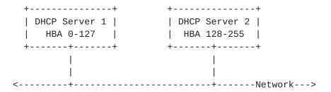
In this example, rather than both servers servicing all clients, each services appropriate half the clients and each services the same set of clients consistently. A redundant set of servers could be added (each configured with appropriate HBAs).
