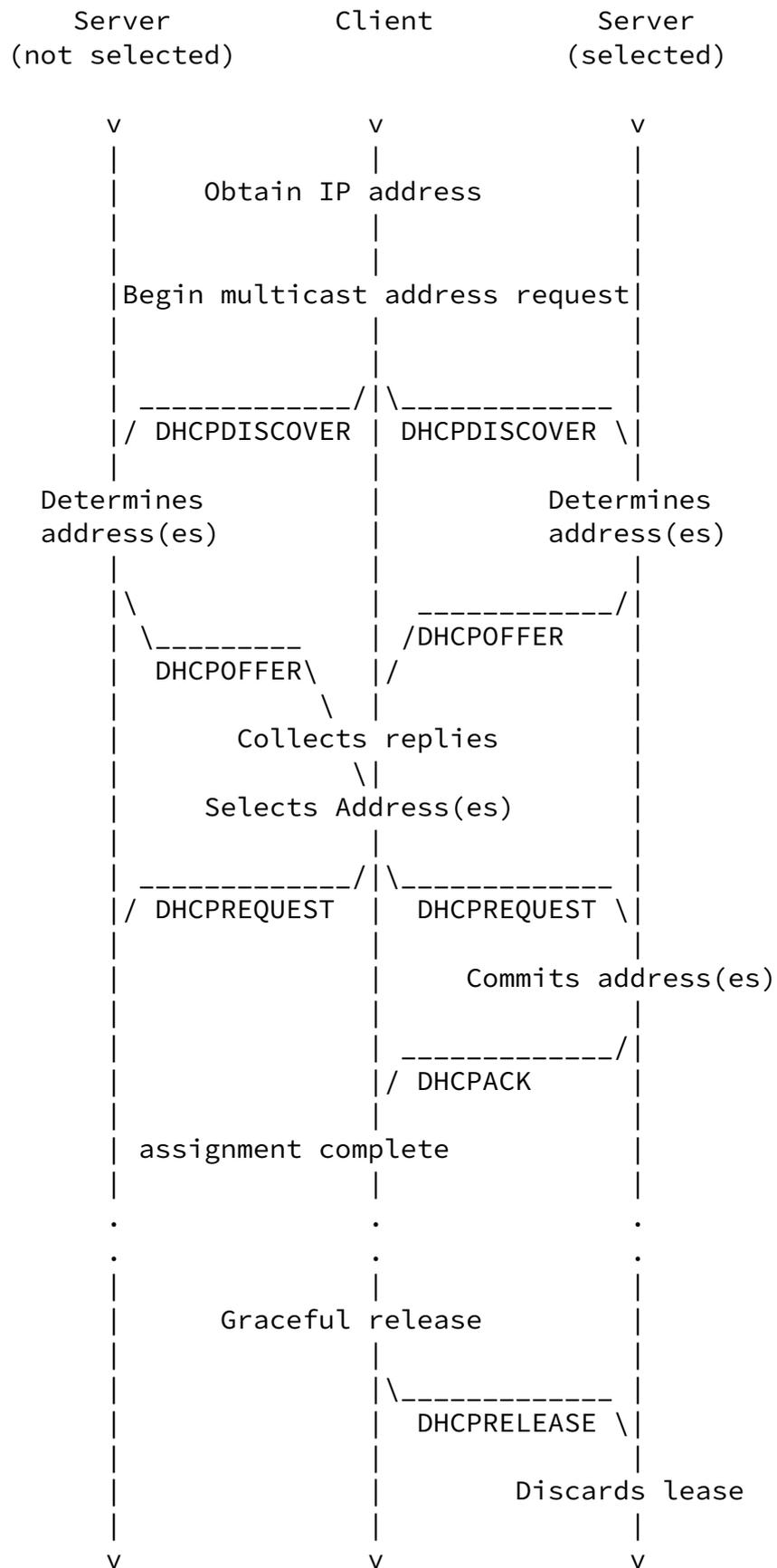
Figure 2: Timeline diagram of messages exchanged between MDHCP client and servers when allocating multicast address(es) using group multicast address for MDHCP capable servers.
