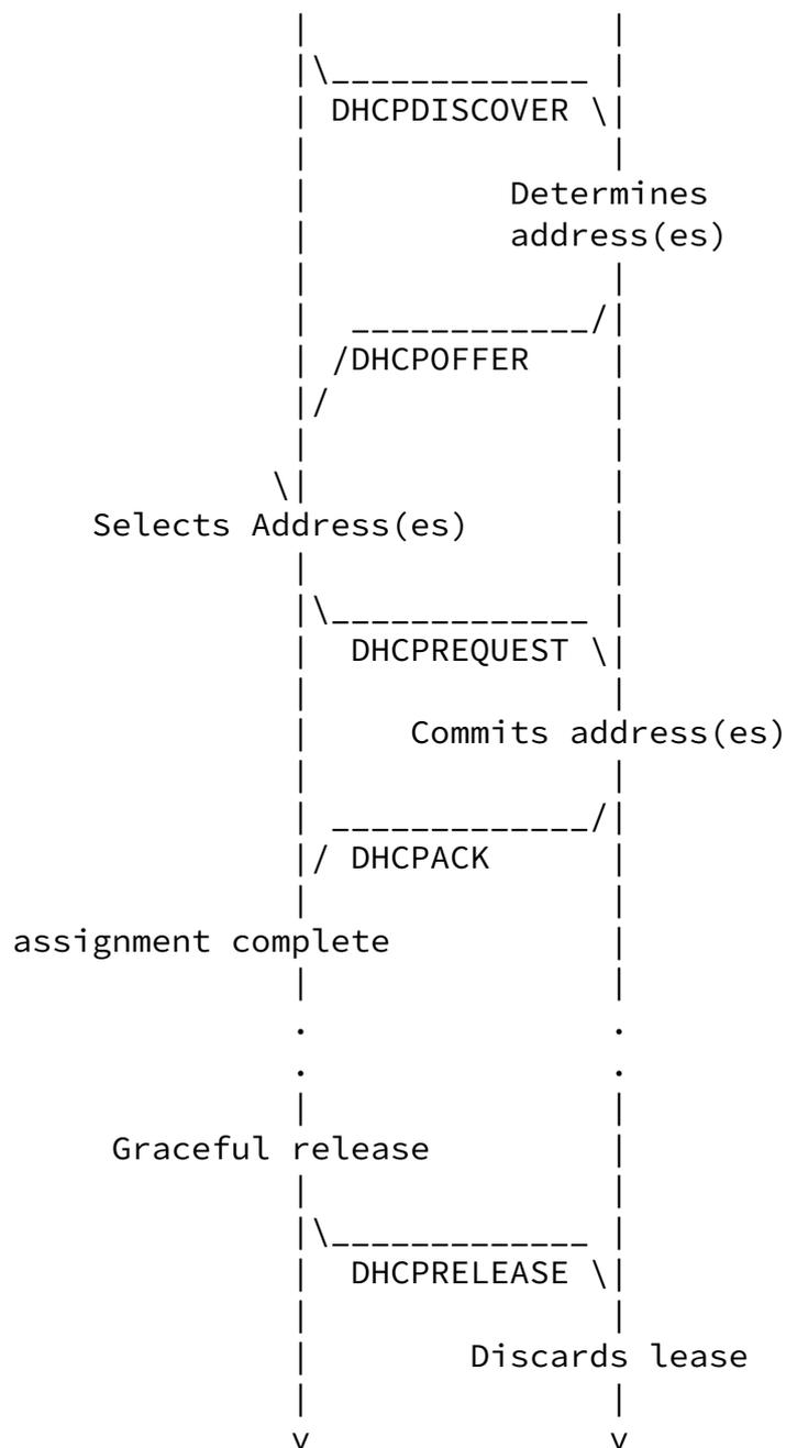
Figure 1: Timeline diagram of messages exchanged between MDHCP client and servers when allocating multicast address(es) using unicast messages to a MDHCP capable server.
