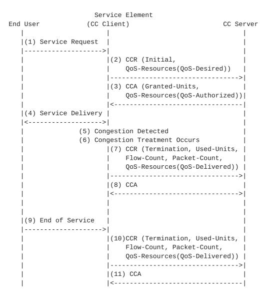
Figure 1: Example of a Diameter Credit Control with Congestion Information
