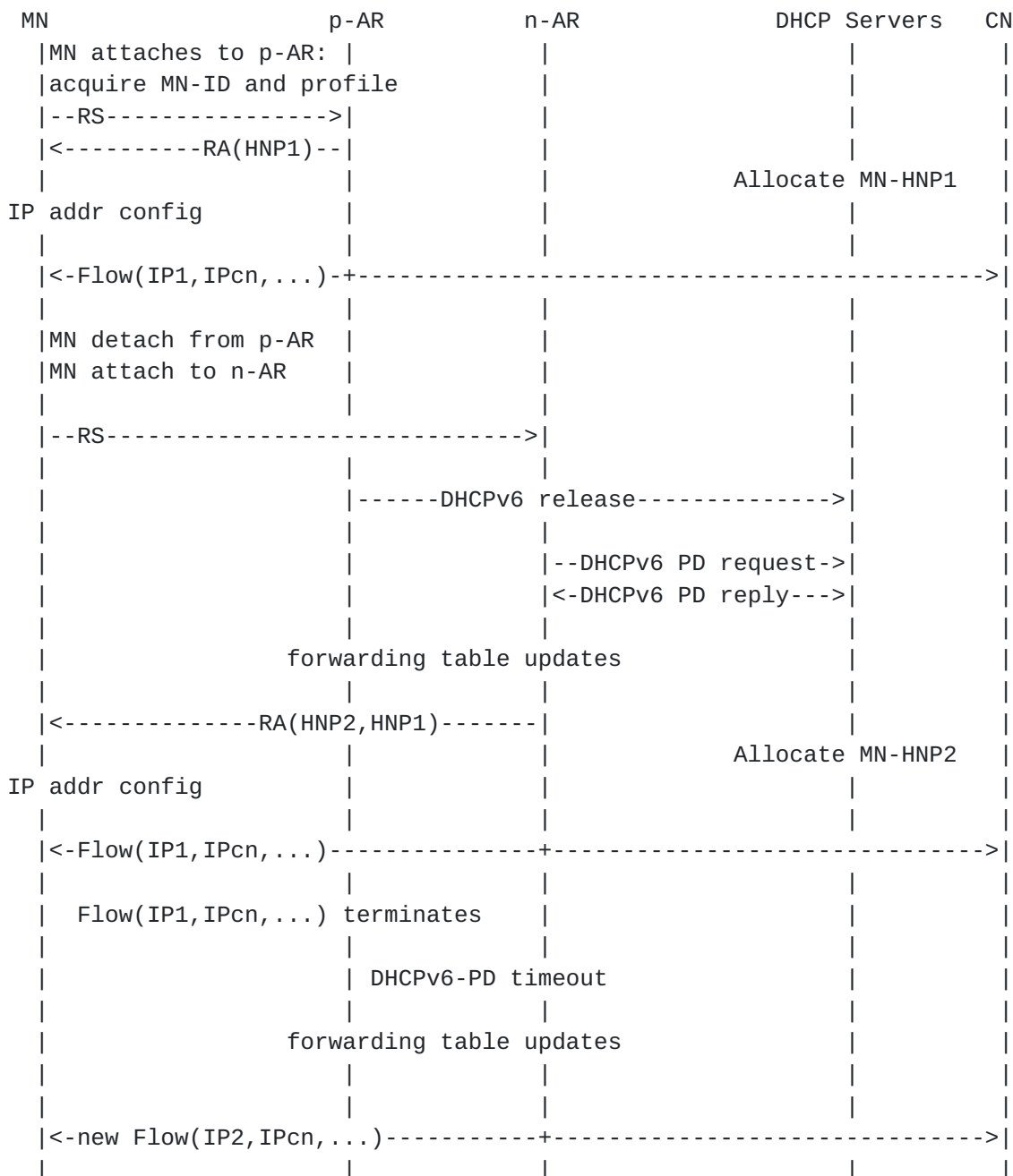
Figure 8. DMM solution. MN with flow using IP1 in Net1 continues to run the flow using IP1 as it moves to Net2.
