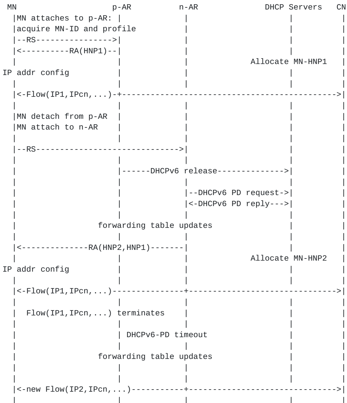
Figure 9. DMM solution. MN with flow using IP1 in Net1 continues to run the flow using IP1 as it moves to Net2.
