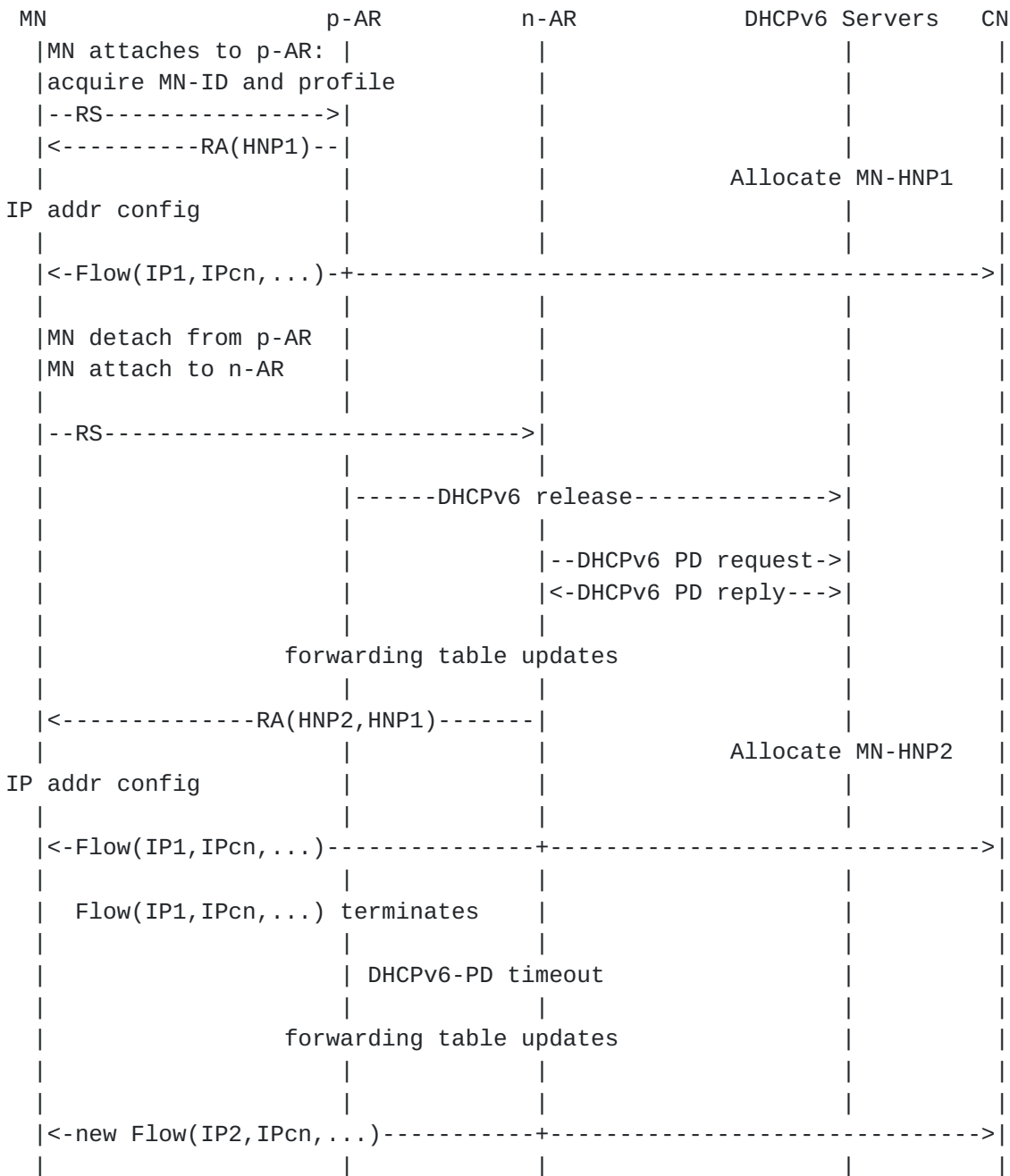
Figure 10. DMM solution. MN with flow using IP1 in Net1 continues to run the flow using IP1 as it moves to Net2.
