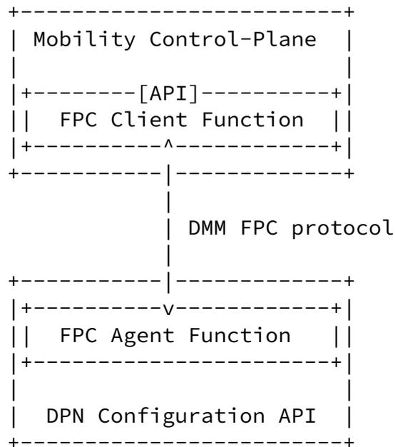
Figure 2: Illustration of the functional reference architecture for DMM Forwarding Policy Configuration (FPC)
