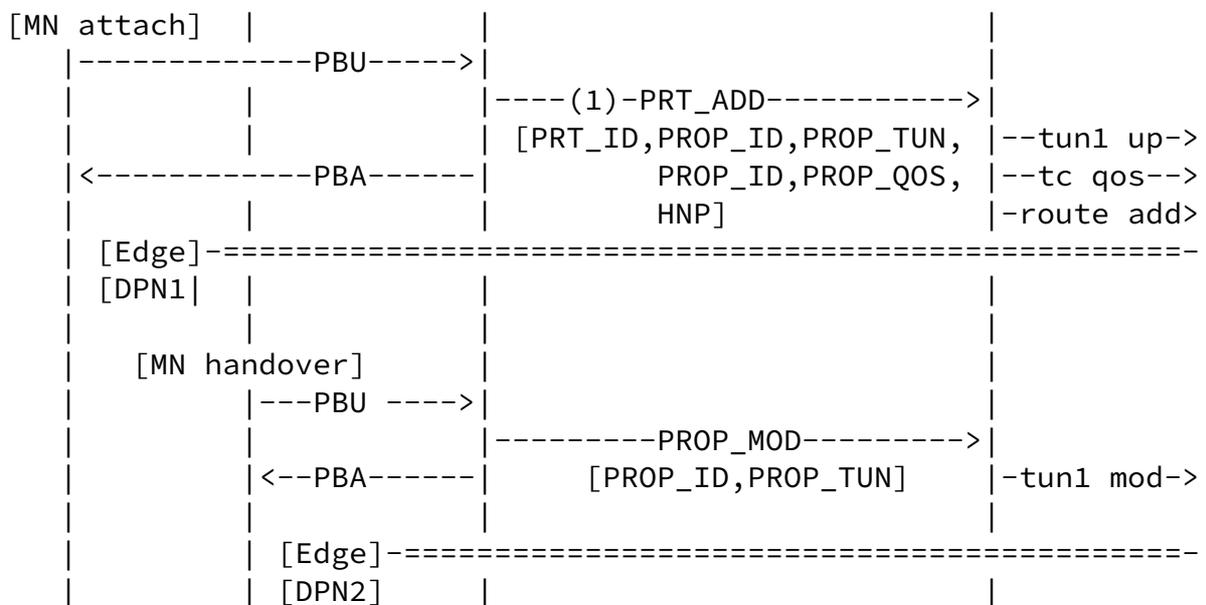
Figure 9: Example: Sequence for Message Aggregation (focus on FPC reference point)
