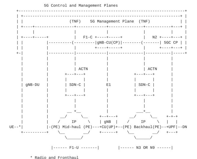
Figure 1: Backhaul and Mid-haul Transport Network for 5G
