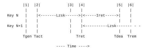
Figure 2: Timeline for a Double-Signature ZSK rollover.
