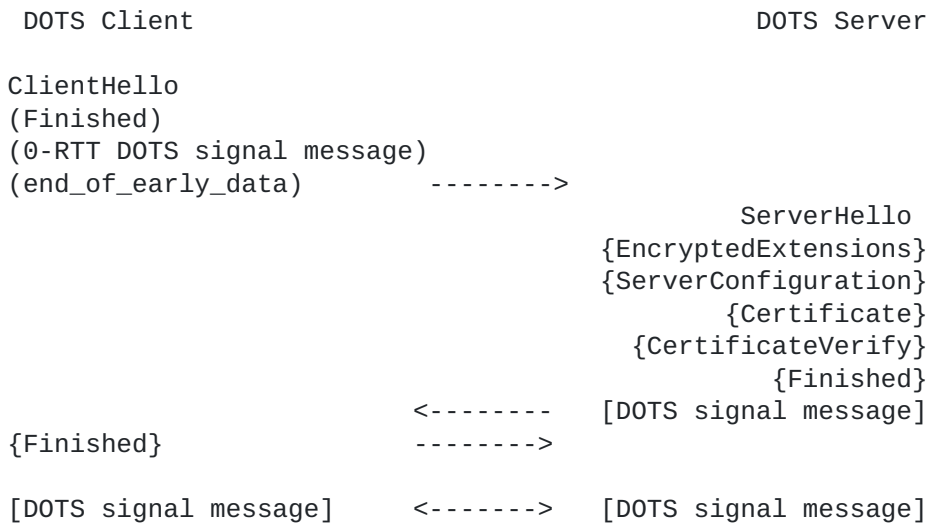
Figure 24: TLS 1.3 Handshake with 0-RTT
