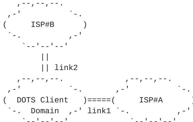
Figure 14: Multi-Homed DOTS Client Domain
