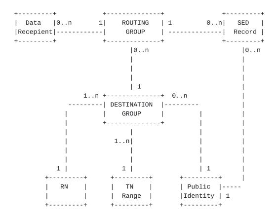
Figure 3: Data Model Diagram
