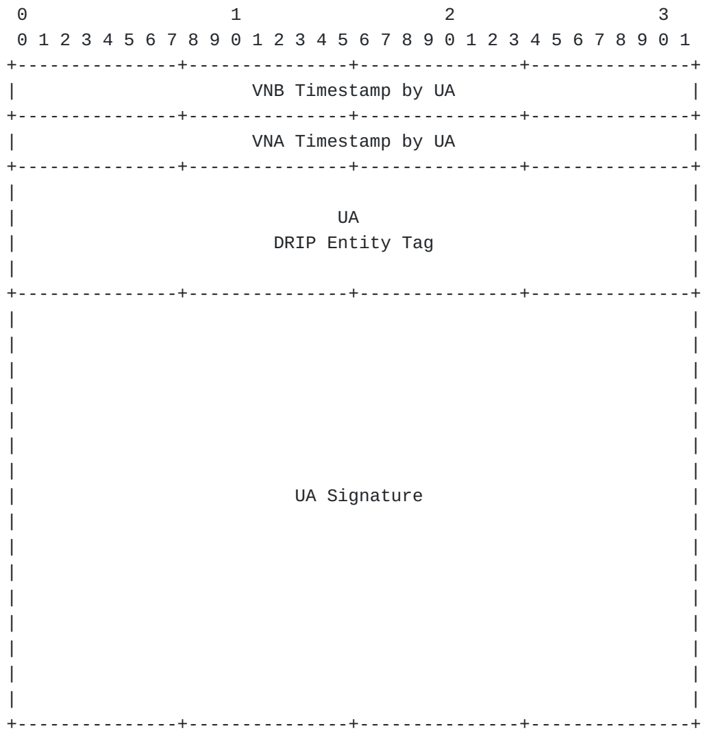
Figure 7: DRIP Wrapper over Extended Transports
