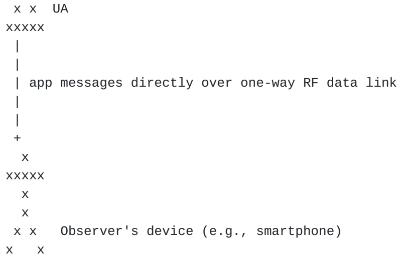
Figure 4: "Broadcast RID Information Flow"
