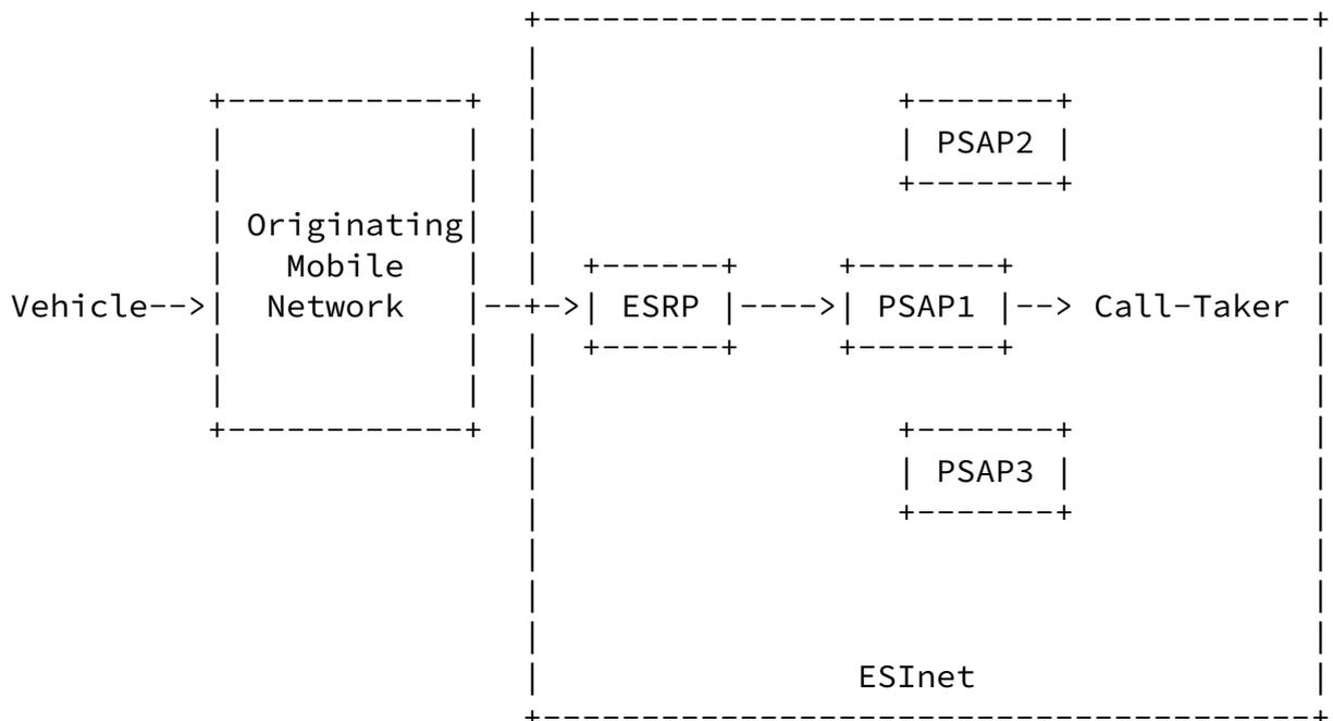
Figure 10: Example of Vehicle-Placed Emergency Call Message Flow
