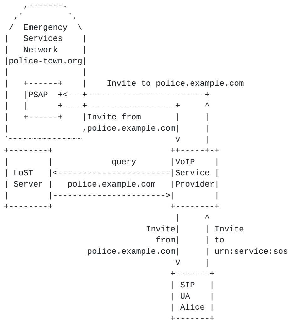
Figure 4: Example for Network-based Service URN Resolution
