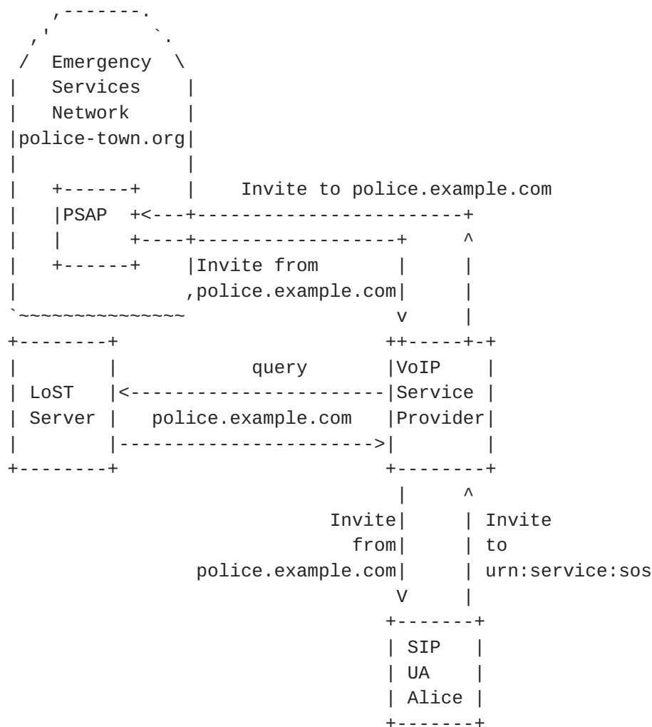
Figure 4: Example for Network-based Service URN Resolution
