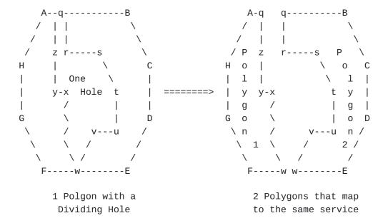
Figure 4: Correct Specification of Hole with Multiple Outer-Boundary Intersections
