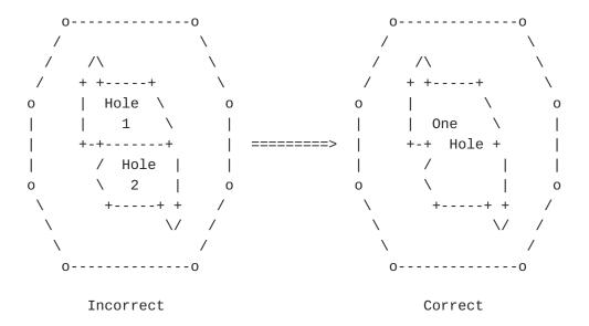
Figure 2: Incorrect Hole Specification with Boundary Sharing
