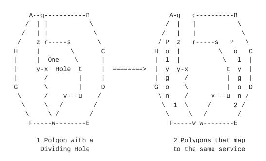
Figure 4: Correct Specification of Hole with Multiple Outer-Boundary Intersections
